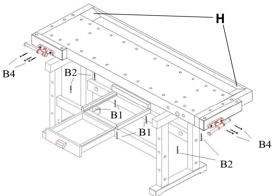
**Important!** Wedges for tool well are supplied separately (part H). Producer recommends to add wedges after approx. 4 weeks. Workbench needs to adapt to the surrounding conditions. In case of need adjust the size of wedges by size of tool well.
