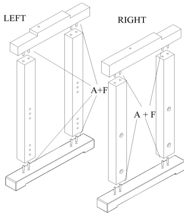
!!! HINT 1 !!! - don't fill up holes for dowels by glue. Smear dowels by glue and insert them into holes.
