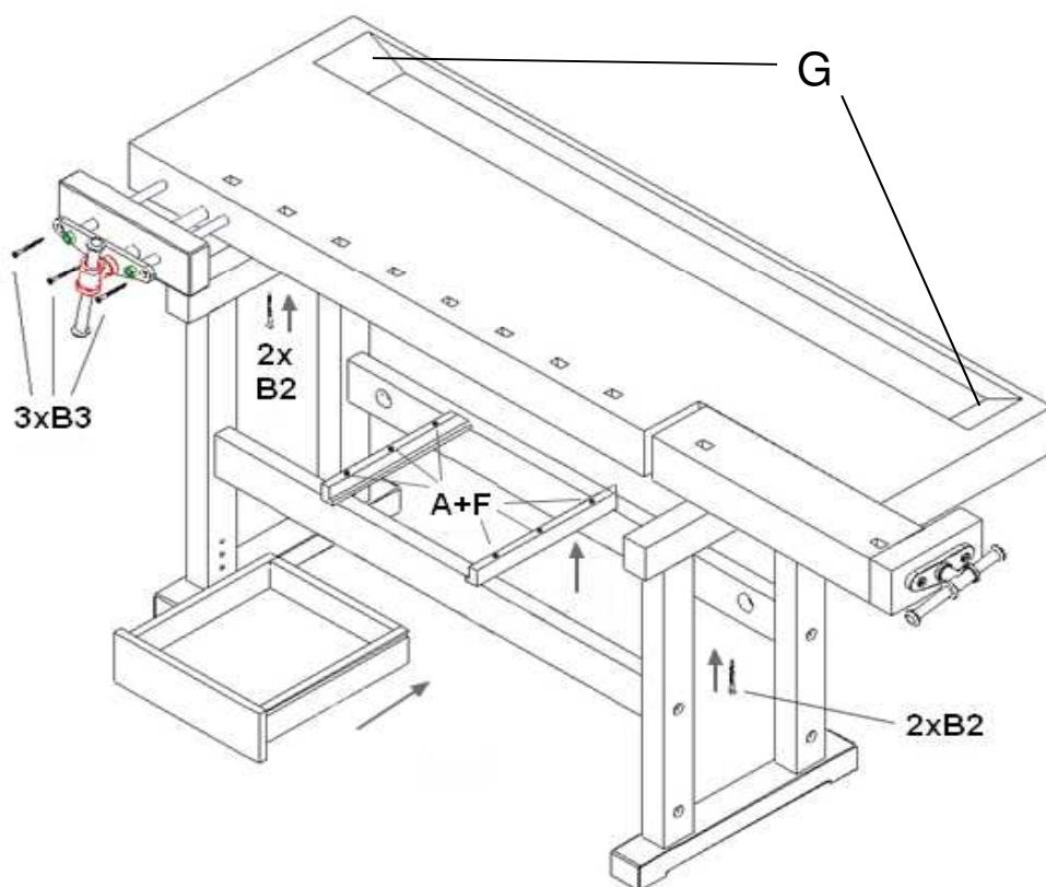
**Important!** Wedges for tool well are supplied separately (part G). Producer recommends to add wedges after approx. 4 weeks. Workbench needs to adapt to the surrounding conditions. In case of need adjust the size of wedges by size of tool well.
