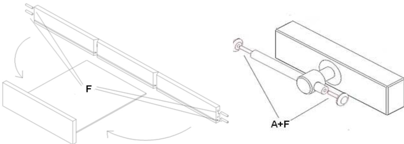
!!! HINT 1 !!! - don't fill up holes for dowels by glue. Smear dowels by glue and insert them into holes.
